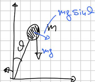
Equation of motion:  $m \ddot{\vartheta} = mg \sin \vartheta \approx mg \vartheta$
