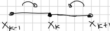
$$\frac{\partial}{\partial t} x_k(t) = \alpha \frac{(x_{k+1}(t) - x_k(t)) + (x_{k-1}(t) - x_k(t))}{l^2}$$
